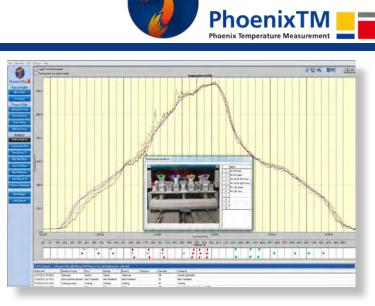
The temperature profile is displayed in the graphics window of the Thermal View software. Thermocouple profiles can be switched on or off individually and you can zoom in for more detailed analysis.
