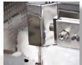
Integral logger tray provides quick and easy data logger installation.
