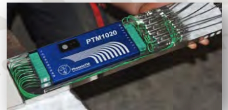
Integrated logger tray with thermocouple clamps for ease of data logger installation and removal
