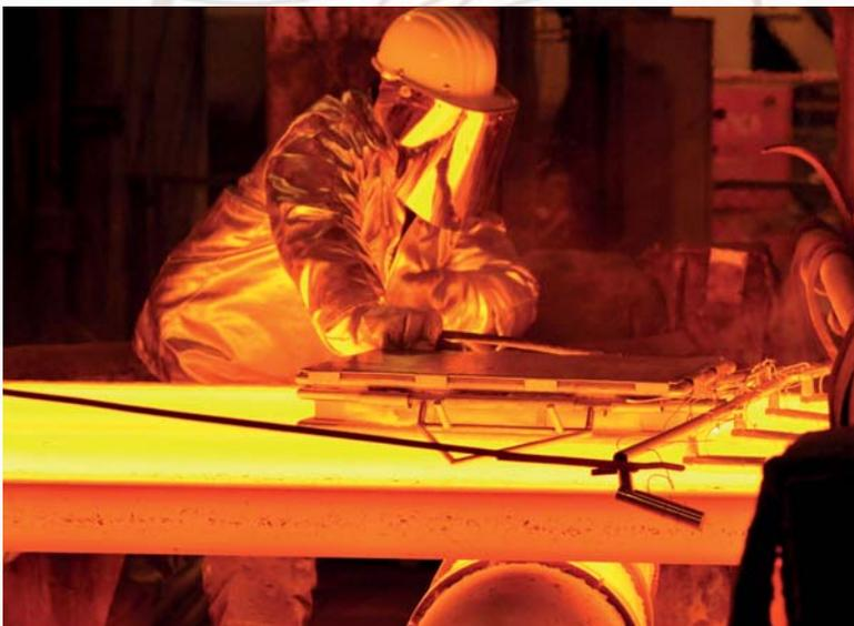
The TS07-100 Thermal Barrier System is specifically designed for Mini-Mill (CSP) applications. It provides thermal protection for the data logger combined with a support arm for the thermocouples measuring both surface and atmosphere temperature. After preparation the system is lowered onto the moving slab using the foldable suspension arms by an overhead crane. When positioned on the slab the arms are lowered to ensure the low height profile of the system is maintained.
