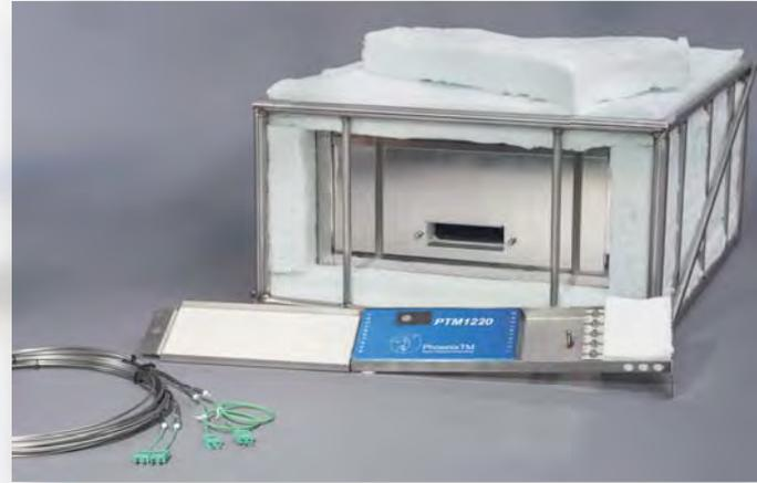
Developed from many years of experience the TS07 has many features specifically for this harsh environment. The data logger fits into an inner tray providing extra protection for the connections whilst clamping thermocouples to ease handling.
